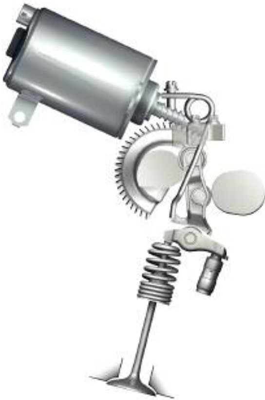
Valvetronic II at minimum valve lift
